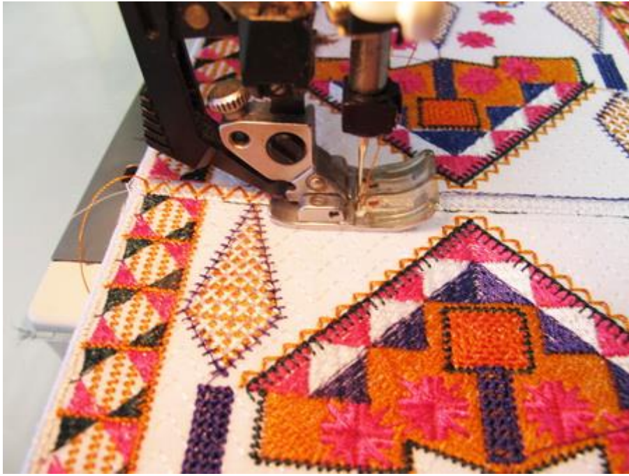
Showing you the stitching over the satin stitch using a triple zigzag stitch from your decorative stitches in your sewing machine
